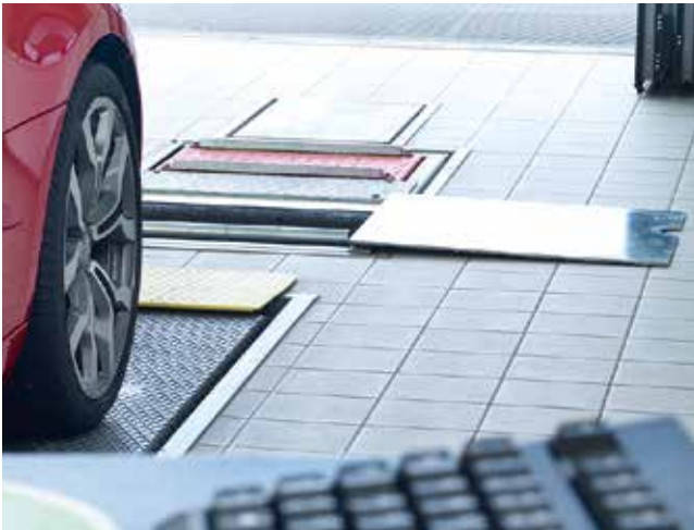
Roll-over protection by means of swivel-mounted roller cover plates
