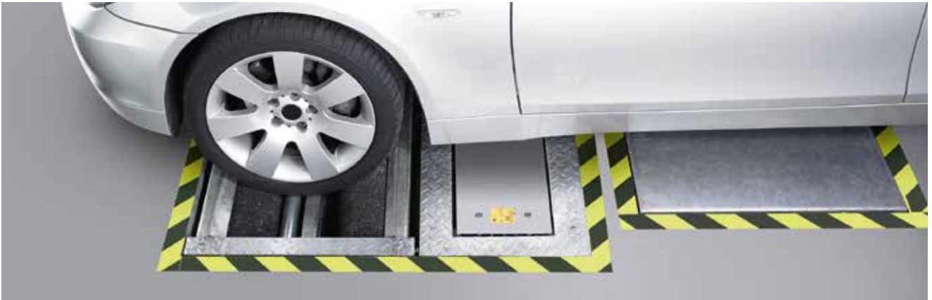
Brake test at the test lane with EUSAMA suspension tester
