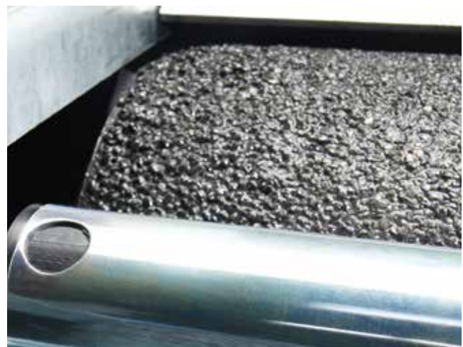
Wear-resistant rollers coated with plastic/corundum
