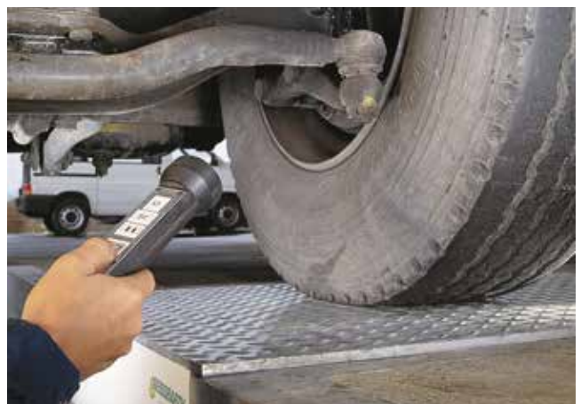
The control lamp combines the function of a torch with a practical control panel.
